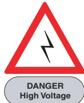
**Switch off the drive for at least 10 minutes before disconnecting, or connecting the motor.**
