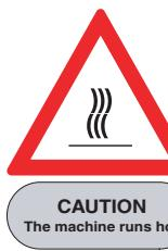
**During operation the motor surface temperature may exceed 100°C. Ensure that temperature sensitive devices do not touch the motor surface.**
