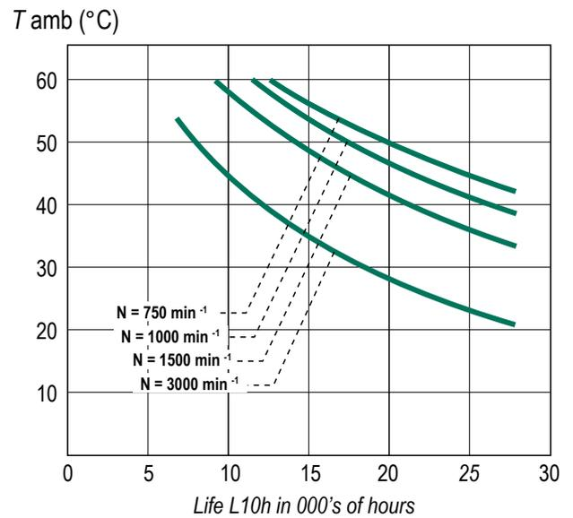
**Bearings with grease nipples**
