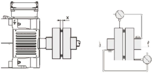
The deviations registered by either shaft will indicate the need for an axial or radial adjustment if the deviation exceeds 0.05 mm.
